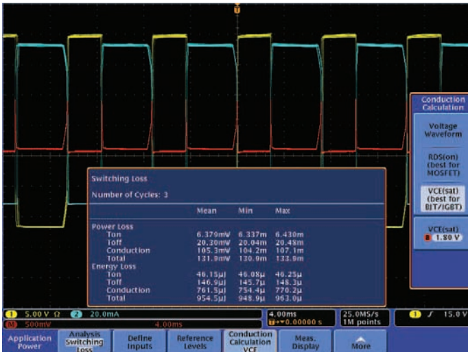
Figure 13. DPOxPWR Switching Loss Measurements on an IGBT.
