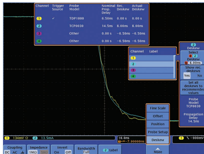
Figure 6. Nominal Correction of Timing Skew between Voltage and Current Probes.
