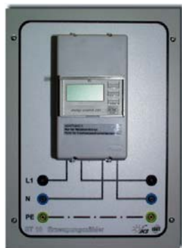
ST 10 Electronic AC electricity mete 1x input, 1x output
