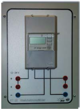
ST 23 Electronic DC electricity meter, 1x input, 1x output
